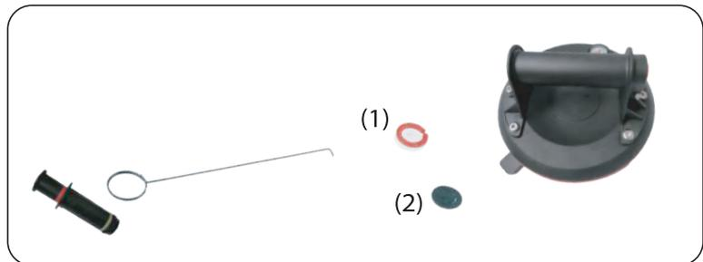
2. Using the hook, pull out the retaining ring (1) of the suction cup body. Take out the rubber valve and check if it is damaged. If so, then insert a new one (2). Finally insert the retaining ring and the piston pressure pump.
