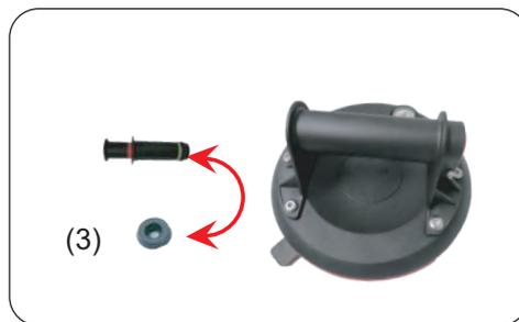
2. Loosen the bolt from the piston body, remove washer, replace the sealing ring (3). Insert the washer and secure with the screw
